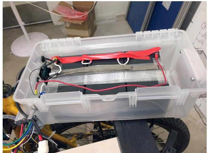
Fig. 38: Batteries Installed in Battery Box
