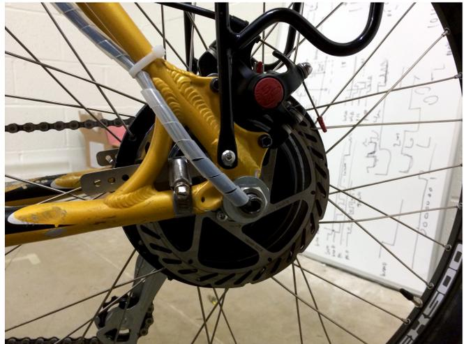
Fig. 51: Detailed View of Disc Brake Installation of Hub Motor
