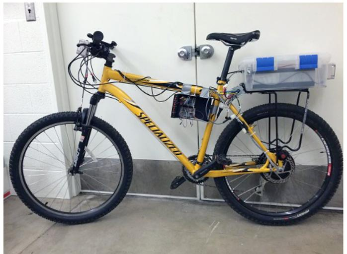
Fig. 35: Specialized Rockhopper with Systems Installed
