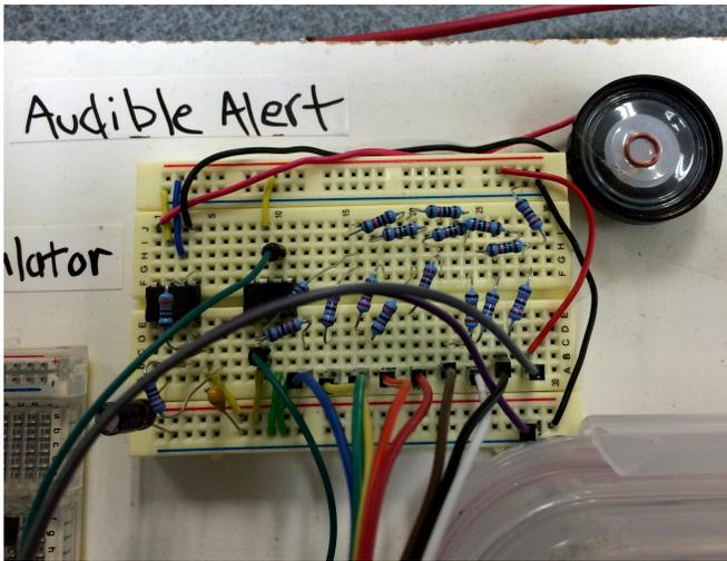
Fig. 16: Breadboard Version of Audible Alert
