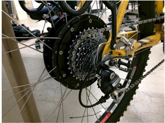
Fig. 50: Detailed View of Drivetrain Integration and Torque Arm Installation
