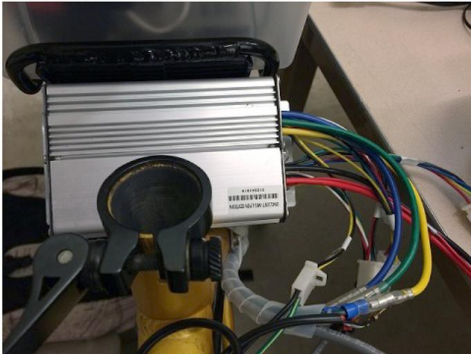
Fig. 37: Lyen 9 FET Mark II Sensored ESC
